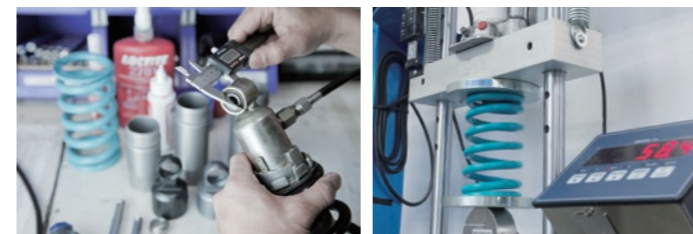
OEM shock dimension, damper characteristic, and other data is being taken.
