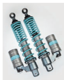
PCX/ADV150 upside down shock shape. Equipped with special clevis (mounting part) without a spherical bearing.
