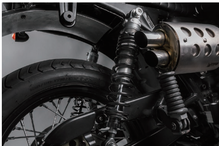
NITRON STEALTH TWIN R3 Series JPY ¥189,000 TST02RS Equips 3way damping adjusters / Remote reservoir tank model
